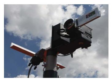
Quick release plate for the camera to allow for easy setup, and protection T-bar to allow you to set the ROVERCAM 17 down on the ground!
